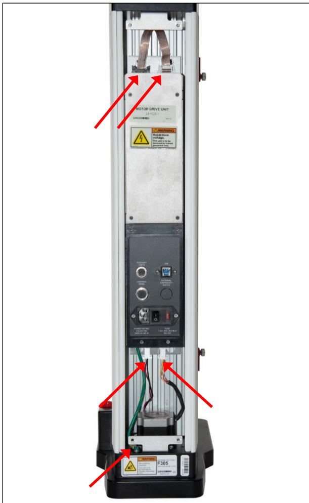
Locations of connectors, ground wire, and bracket
