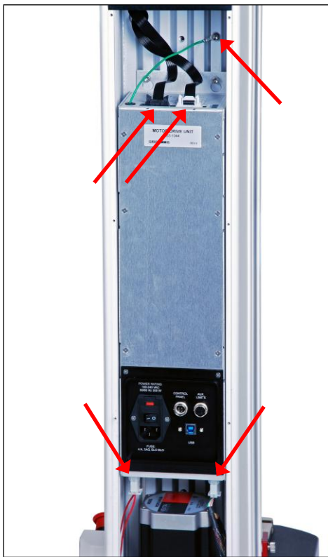
Locations of connectors and ground wire
