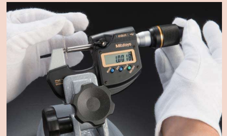
Recommended micrometer stand: 156-101-10
