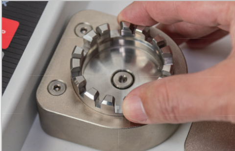
▲ The standard adjustable wire terminal fixture accommodates wire diameter sizes up to AWG 3 (0.25 in [6.3 mm]).
