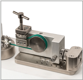
AC1134 Bollard grip assembly Secures the free end of the sample via a bollard and vise. Based on the model G1102 grip.
