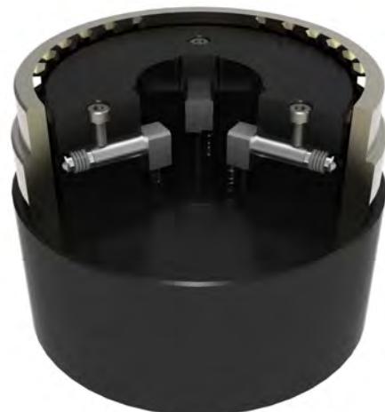
APPLICATION: DZ PROBE CHECKING ID OF RING
