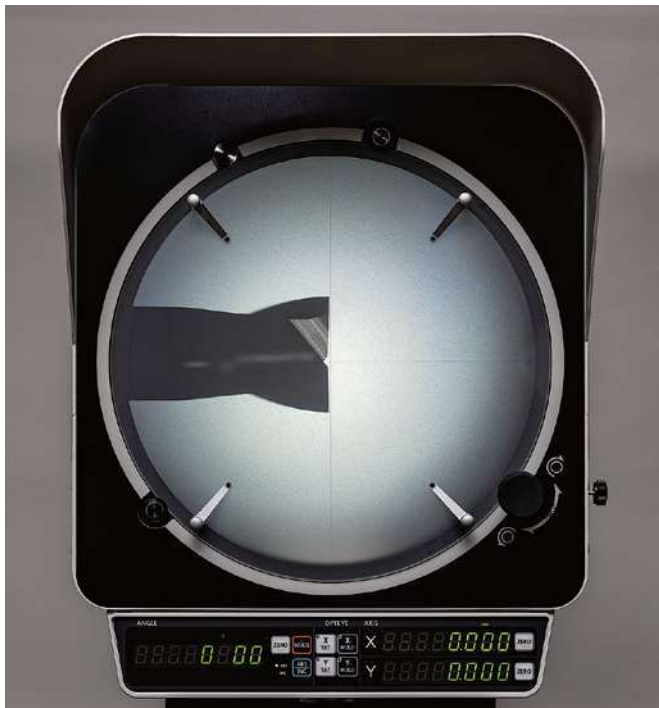
Example of attaching the LED circular illuminator on PJ-PLUS
