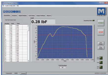
↗ View real time data in graphical and tabular formats. Also, remotely zero the force gauge or test stand travel display.
