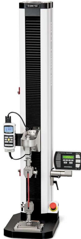
ESM750 750 lbF [3.4 kN] 32 in [813 mm] travel
