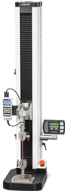
ESM1500 1,500 lbF [6.7 kN] 32 in [813 mm] travel
