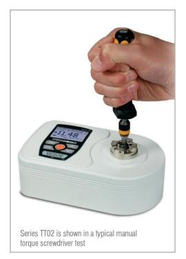
Series TT02 Torque Tool Testers present a simple and accurate solution for testing manual, electric, and pneumatic torque screwdrivers, wrenches, and other tools. These testers are compact and rugged, suitable for production environments. A universal 3/8" square receptacle accepts common bits and attachments. The TT02 captures peak torque in both measurement directions, and also calculates 1st and 2nd peaks, useful for click-type tools.
