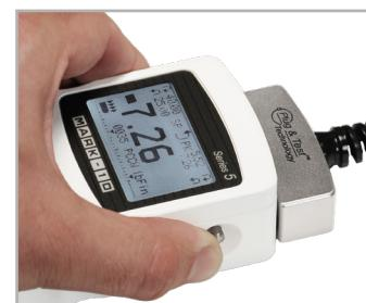
The Plug & Test® connector locks into the receptacle in the indicator when fully inserted. Dual buttons on the indicator housing release the connector for easy removal. Gold plated spring contacts ensure long lasting and reliable connection.
