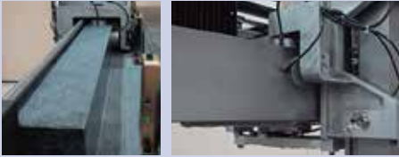
Integrated Y-Axis in Granite Table
